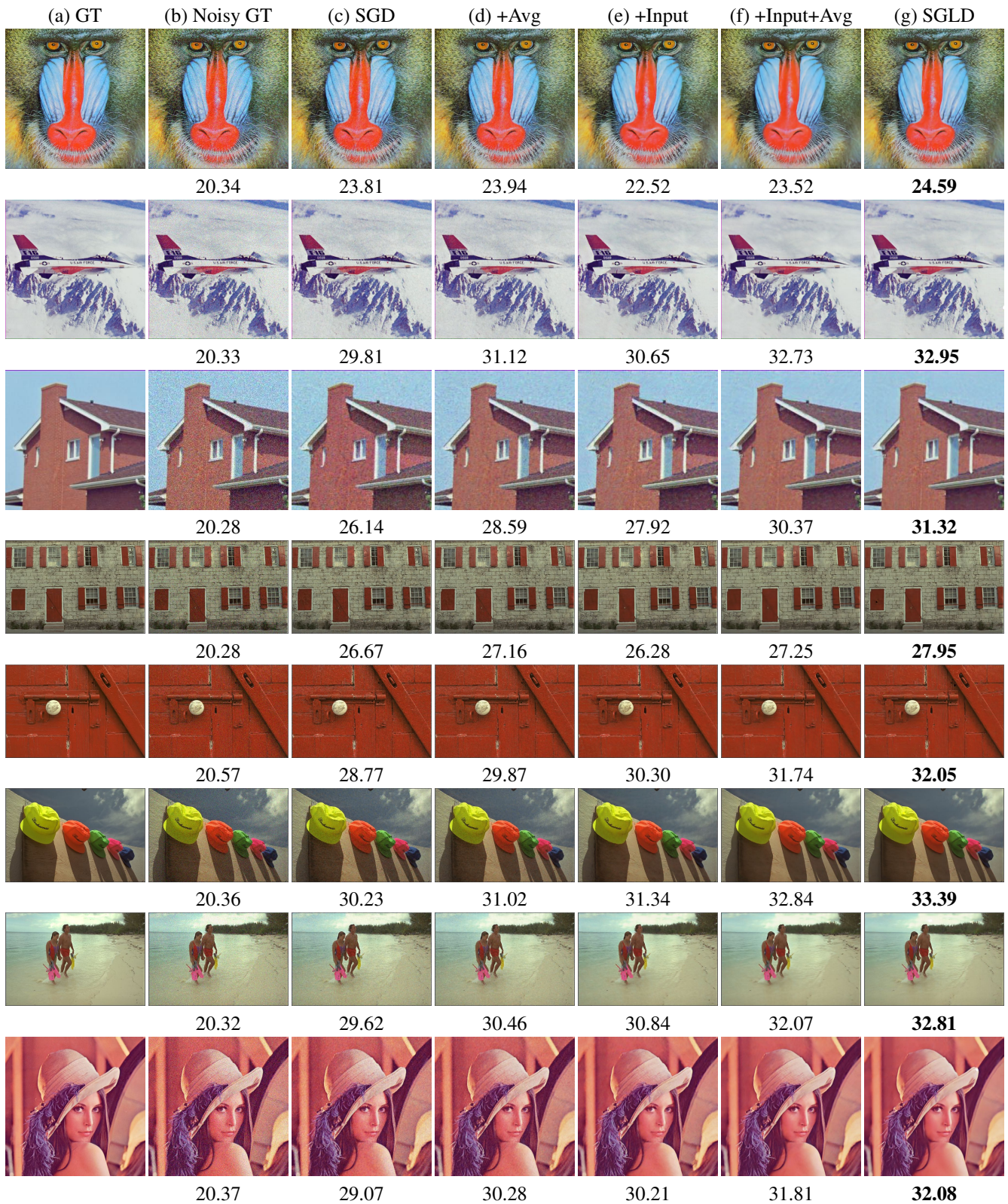
Figure 1. (Best viewed magnified.) Comparison of inference schemes for image denoising. From left to right each column shows (a) ground truth image, (b) the ground truth image corrupted with Gaussian noise of \sigma = 25 , (c) inference with SGD and early stopping (iteration picked at maximum PSNR), (d) previous step with exponential window average, (e) SGD with input noise and early stopping, (f) the previous procedure with exponential window averaging, and (g) SGLD. Underneath each figure the PSNR values are listed. Note that except SGLD every procedure requires early stopping.
