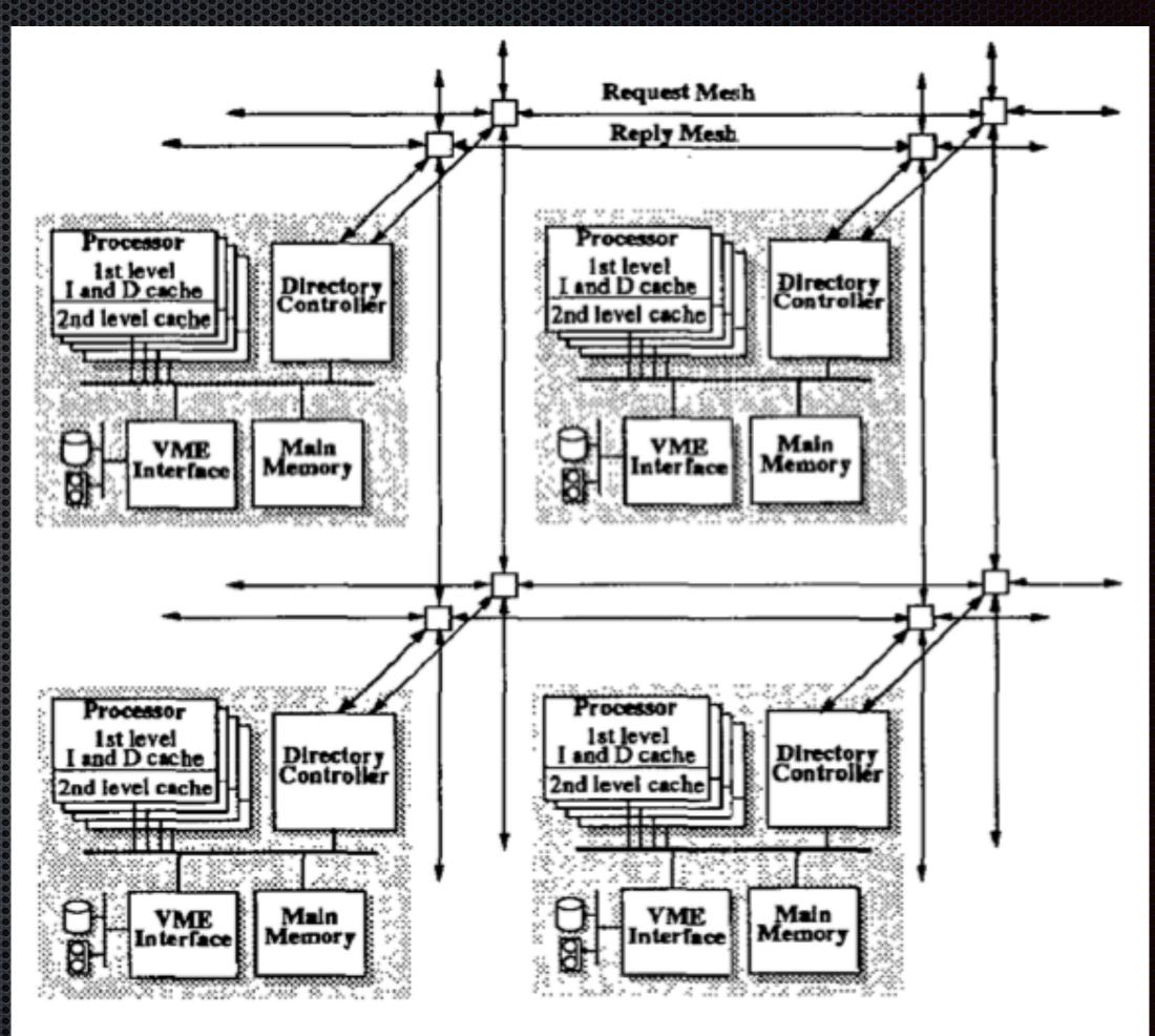
Figure 2: Block diagram of sample 2 x 2 DASH system.
