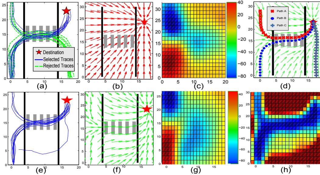
Figure 1: (a) Plan view of zebra-crossing with the path traces of simulated pedestrians using it to get from one sidewalk to another. (b) Prior navigational map. (c) Predictive mean of the deviation function. (d) Posterior map with 3 sample trajectories generated from different starting locations. (e) Path traces with added jaywalker. (f) Updated posterior navigational map. (g) Updated predictive mean. (h) Updated predictive variance.
