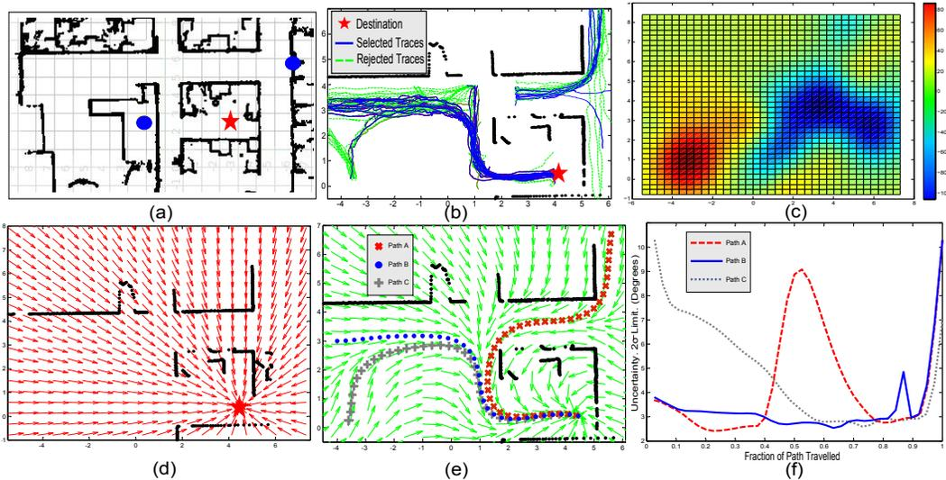
Figure 2: (a) Occupancy grid of office area - positions of laser rangefinders marked in blue. (b) Path traces of pedestrians detected by lasers. (c) Predictive mean function of  $\Psi$ . Sparsely sampled quiver plot of the prior (d) and posterior (e) navigational maps with examples of resulting routes to the destination taken from three different starting locations using the latter. (f)  $2\sigma$  boundary (degrees) vs. fraction of route travelled for each sample route.
