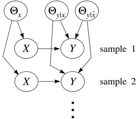
Figure 4: A Bayesian-network structure depicting the assumption of parameter independence for learning the parameters of the network structure  $X \rightarrow Y$ . Both variables  $X$  and  $Y$  are binary. We use  $x$  and  $\bar{x}$  to denote the two states of  $X$ , and  $y$  and  $\bar{y}$  to denote the two states of  $Y$ .
