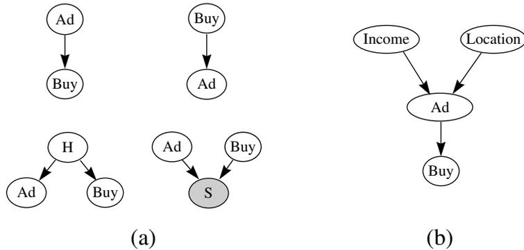
Figure 9: (a) Causal graphs showing for explanations for an observed dependence between *Ad* and *Buy*. The node *H* corresponds to a hidden common cause of *Ad* and *Buy*. The shaded node *S* indicates that the case has been included in the database. (b) A Bayesian network for which *A* causes *B* is the only causal explanation, given the causal Markov condition.
