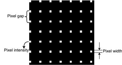
Figure 2: Our backdoor trigger has three parameters: pixel intensity  $\alpha$ , pixel gap  $g$ , and pixel width  $w$ . For presentation clarity, we use high pixel intensity here, but in experiments we use low intensities to ensure attack stealth.
