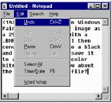
Cut and Copy are gray because *nothing is selected*, and so nothing can be cut or copied at the current time. (The cursor is just after the question mark on the last line of the image, and does not cover any characters. It has zero width.) Note that this question has nothing to do with the clipboard or what is in it right now.
