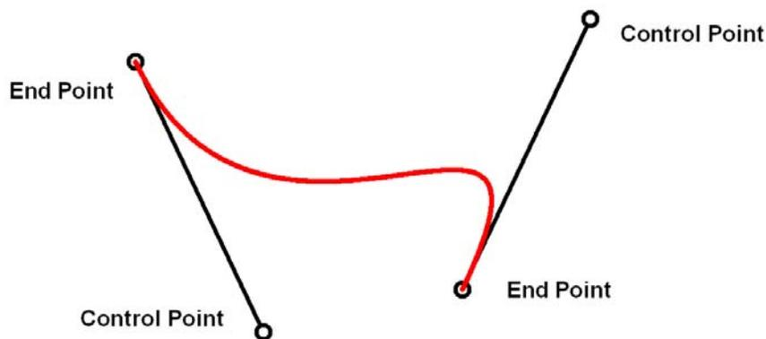
Note that the curve is **tangent** to the control lines at each of the end points, and that the curve falls entirely inside the **convex hull** of the four points (the smallest polygon that surrounds all four points).
