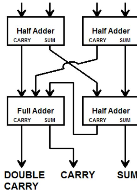
By extending this process even further, we will find that the adders for the partial product columns get more and more complicated. We can extend the quad adder to a “quint adder” by replacing one of the input half adders with a full adder, and then extend it again to a “hex adder” by replacing both of them, as shown below:
