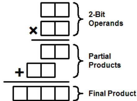
In binary each partial product is generated by multiplying an operand by either 0 or 1, resulting in either zero or a copy of the operand. This is the same behavior as a group of AND-gates. One 2-input AND-gate is used for each pair of bits, then the bits are added together with half-adders and full-adders to generate the final product. The hardware for multiplying two 2-bit numbers together is shown below:
