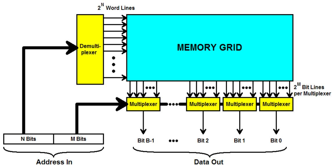
For example, a 64K byte memory system requires 16 address bits and 8 data bits. The grid contains  $2^{16} \times 2^3 = 2^{19}$  data bits. Arranging the memory as 64K rows (word lines) by 8 columns (bit lines) requires a demultiplexer with  $2^{16}$  AND-gates, each with 16 inputs, and no multiplexers. This is 65536 separate AND-gates.
