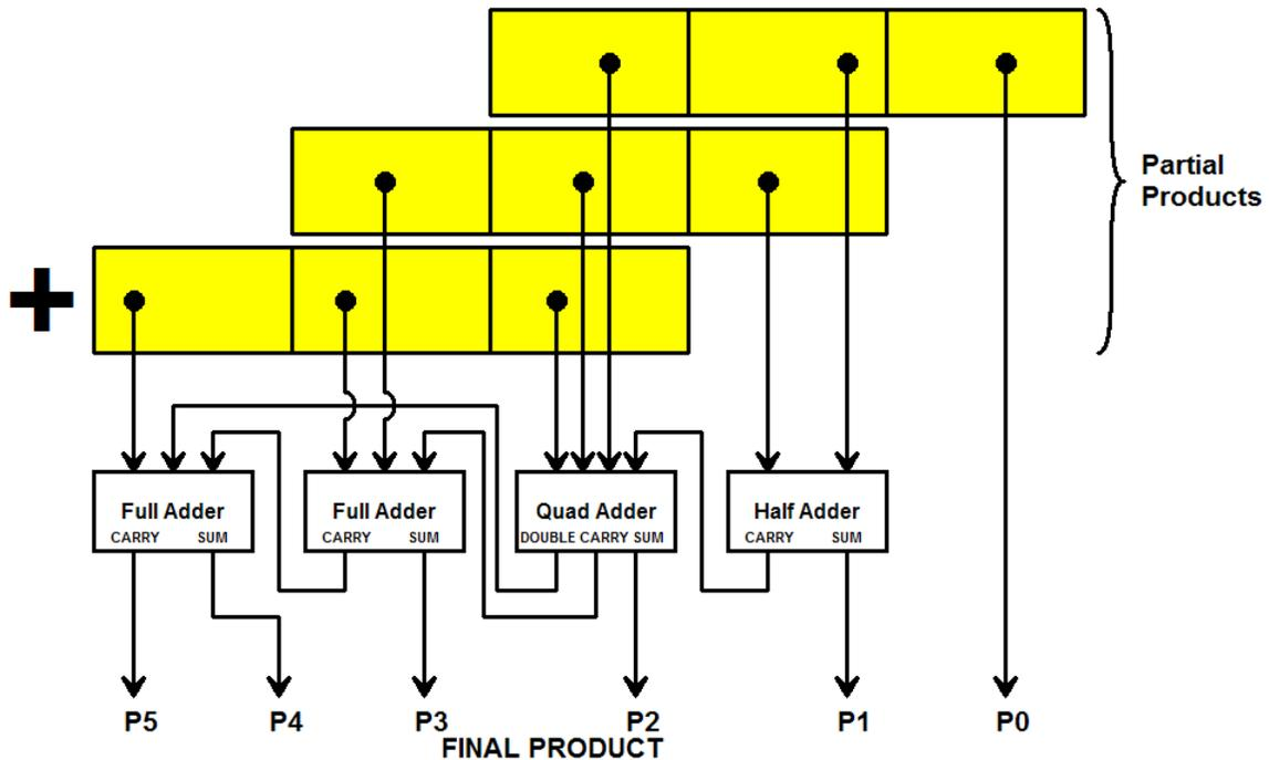
Notice that the quad adder circuit returns a 3-bit sum, emitting the sum bit to the answer, a carry bit to the next stage of partial products, and a *double-carry* to the stage beyond that.
