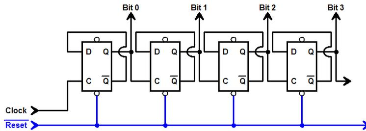
The configuration just described, where the Q-bar output feeds back into the D input, is so common that it has its own symbol. This symbol, shown below, is called a *triggered, toggle*, or T flip-flop. The T input is just a relabeling of the clock input in the D flip-flop, but it indicates that a clock pulse on the T line will cause the outputs of the flip-flop to switch, or toggle, from one state to the opposite state.
