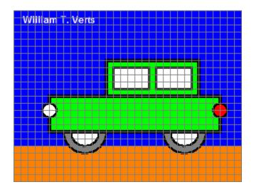
All items are on a 10-pixel boundary. For example, the small white circle that represents the head light is at coordinates <50,140> with a radius of 10 pixels and a **stroke-width** (thickness of the surrounding circle) of 3 pixels.
