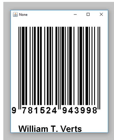
The purpose of your Python program is to let a user enter any number containing up to 13 digits, such as 9781524943998, and then draw out the bar code and text as shown here on the right. If the number contains fewer than 13 digits, enough 0s will be appended to the left to make a total of 13.
