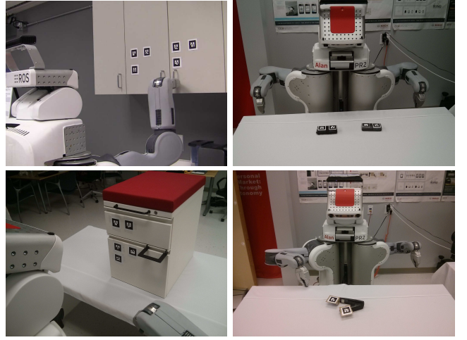
Fig. 6. Four experimental scenarios. Top-left: rotational cabinet door with an incomplete demonstration; top-right: two free-body erasers moved apart in a straight line; bottom-left: locked drawer as a rigid joint; bottom-right: stapler as a rotational joint.
