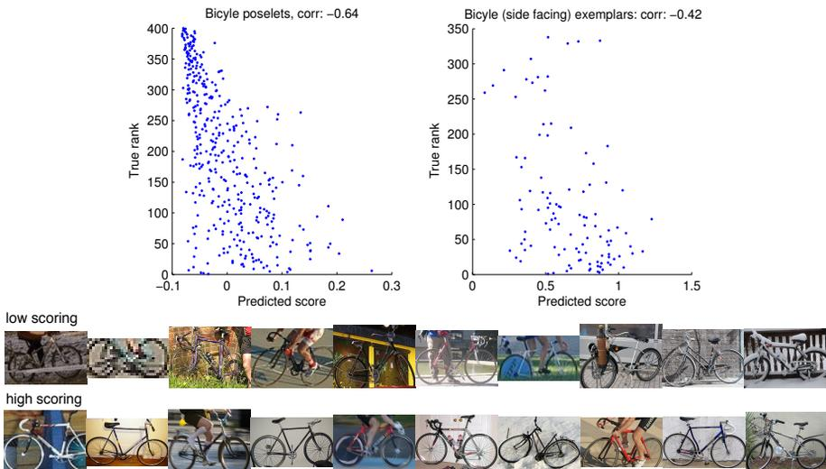
**Fig. 4. An analysis of bicycle filters.** (Top-left) Scatter plot of true ranks and the ranker score of the bicycle poselets. (Top-right) the same for all the exemplars of side-facing bicycles. The high scoring side-facing exemplars (Bottom row) exhibit high contrast and less clutter than the low scoring exemplars (Middle row).
