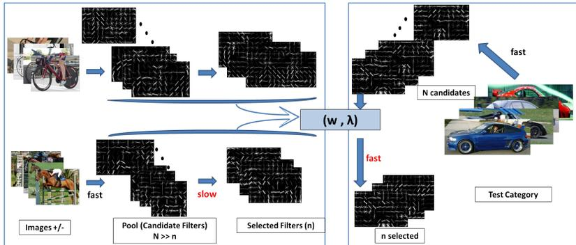
**Fig. 1.** Outline of our approach: Left block shows the training pipeline which is used to obtain a linear ranker ( $\mathbf{w}$ ) and diversity tradeoff parameter  $\lambda$  (described in Sect. 3) on a set of categories. Our system improves the bottleneck of the selection procedure by learning to predict the utility of filters for a new category.
