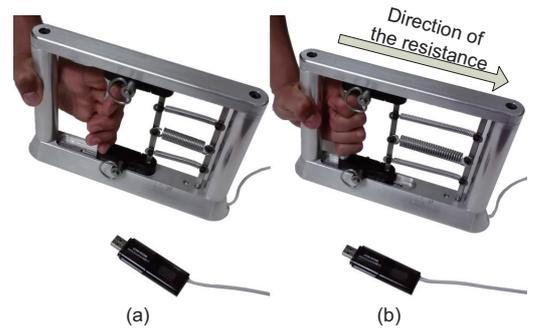
Fig. 1. (a) The digital handgrip device used in its resting position. (b) The handgrip when the handle is moved to its maximum displacement. The direction of the spring resistance is illustrated in arrows.
