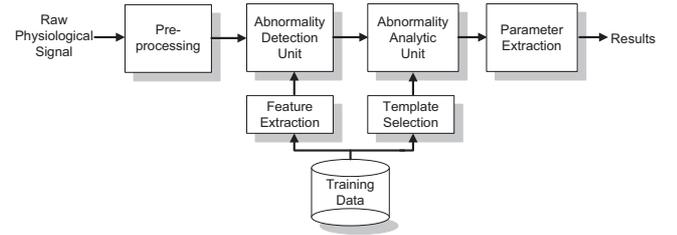
Fig. 4. Graphical overview of the signal processing framework.
