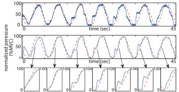
Fig. 5. An example of the results of the pre-processing unit. (Top) The raw input time-series. (Middle) The low-pass filtered time series. (Bottom) The partitioned subsignals representing muscle contraction.
