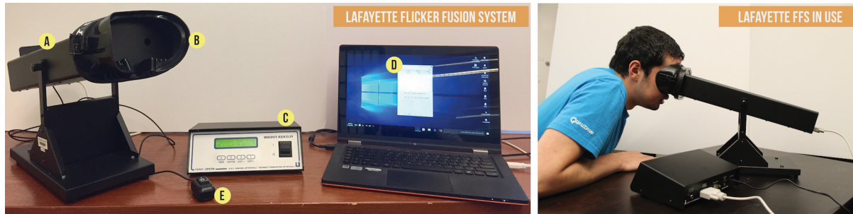
Fig. 4. Left: The Lafayette Flicker Fusion System (Lafayette FFS) has three components: a viewing chamber with the light stimulus (A, B), a controller (C), and a software program to record results (D). The clicker (E) is connected to the viewing chamber and records a person's input (i.e., indicating they see a flickering light or a fused light). Right: To use the Lafayette Flicker Fusion System, a person presses their face against the mask covering the viewing chamber so as not to allow any outside light. The person then focuses on the light inside the viewing chamber and uses the clicker to record their input.
