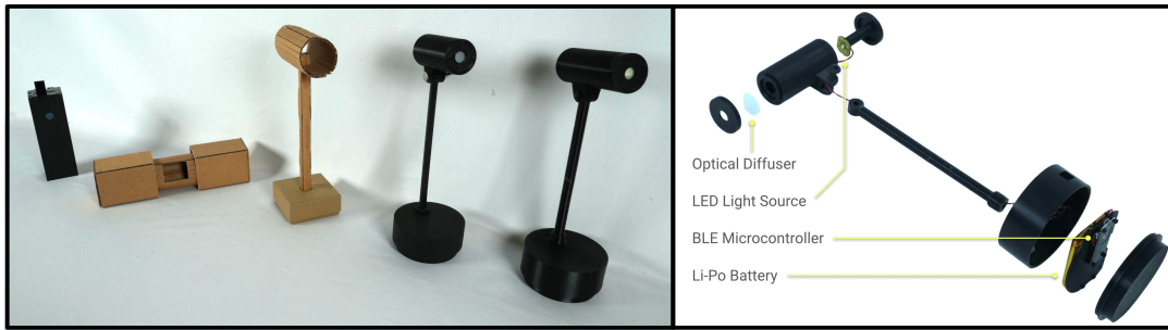
Figure 3: Left: Explorations and iterations in Beacon’s form, from the early prototype developed by Karkar et al. [31] (left-most), through early low-fidelity explorations of potential forms, to development and refinement of Beacon’s current form (right-most). Right: An exploded view of the main components in the current Beacon design. Note the threading designed into each 3D-printed component, allowing parts to be screwed together in assembly, reducing required time and potential error (e.g., glue damage).
