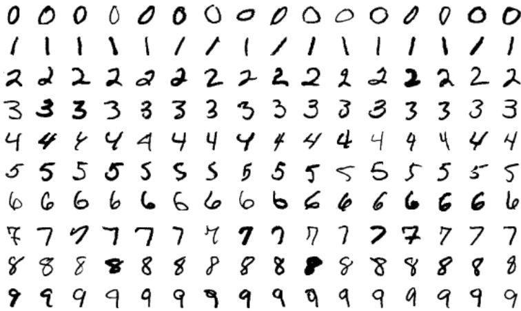
Figure 1.1: Example data that could be provided to the Predict algorithm. Each row corresponds to a different label, from zero to nine. These images are examples of some of the entries in a popular data set called the Modified National Institute of Standards and Technology data set, which is commonly called MNIST (pronounced “em-nist”). If you were standing in for the Predict algorithm and saw the handwritten number below as an input for which you should predict the label, what would you output?
