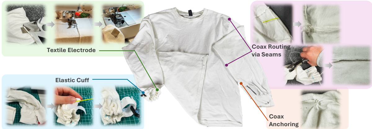
Fig. 6. Design and fabrication of CardioTattoo's customized bridging shirt, achieving appropriate contact with tattoos and smartwatches and low-loss signal propagation, without reducing the softness and flexibility of the garment.
