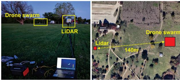
Figure 10: Experimental setup using LiDAR to scan the drone swarm at *Droneshow1*.
