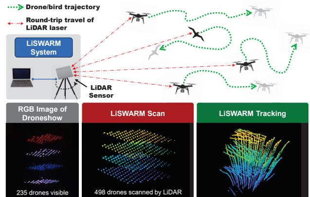
Figure 1: The proposed concept of using low-cost off-the-shelf LiDAR system for drone swarms detection and tracking.
