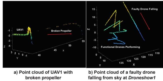
**Figure 24: Recognition of broken propeller in test drone and faulty drone at Droneshow1.**
