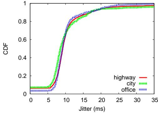
**Figure 4.** CDF of observed jitter (HelixServer using UDP transport)
