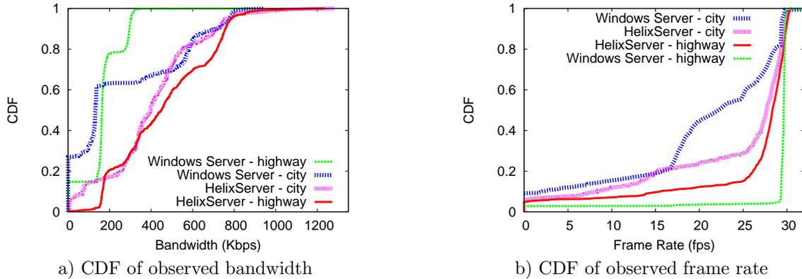
Figure 9. Mobile streaming performance of Windows Media Server and HelixServer
