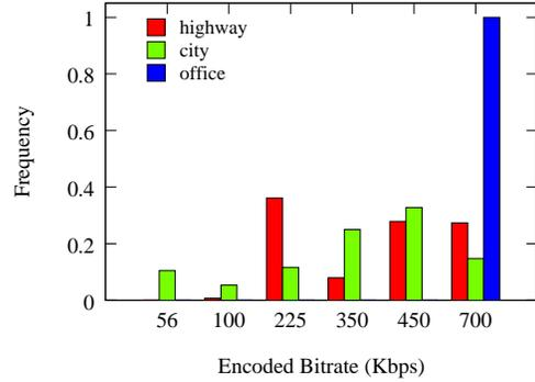
**Figure 3.** Histogram of encoded bitrate (HelixServer using UDP transport)
