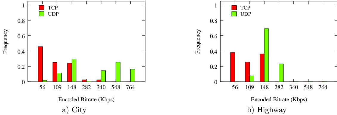
Figure 8. Histogram of encoded bitrate using Windows Media Server
