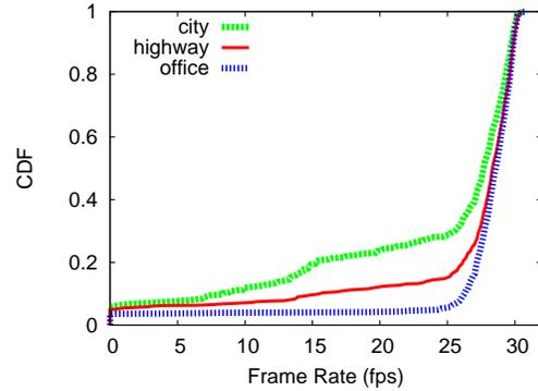
**Figure 5.** CDF of observed frame rate (HelixServer using UDP transport)
