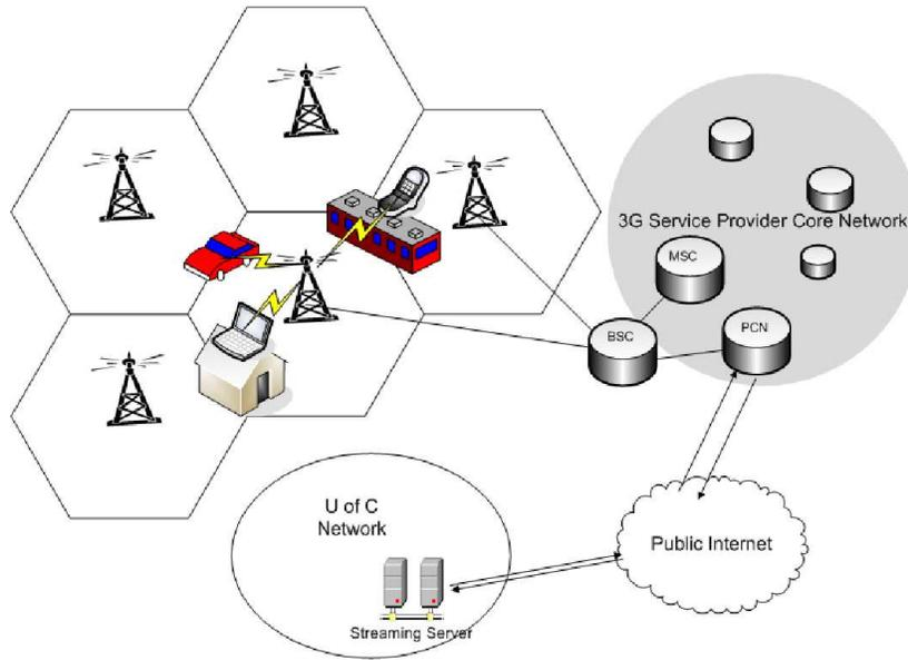
**Figure 1.** Experiment set-up to evaluate streaming performance
