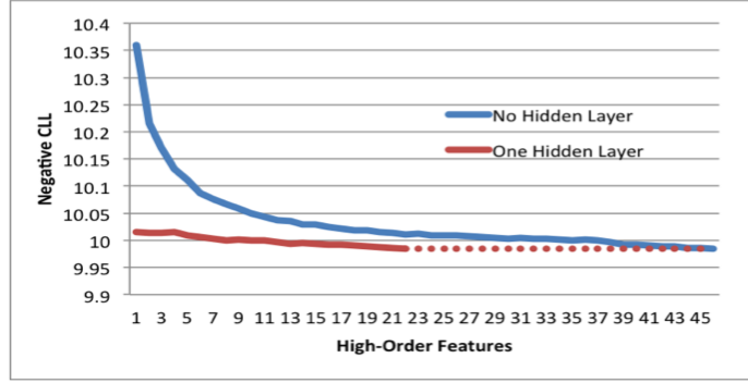
FIGURE 5.2. Trainset negative conditional log-likelihood versus the number of high-order features for GACs with multilayer perceptron with no hidden layer and one hidden layer.
