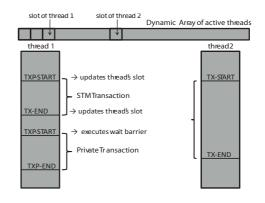
**Figure 2.** Two threads execute transactions. We see the dynamic array used to track quiescing information and bars tracking the execution phases of the two threads. Upon start and finish, the threads update the dynamic array slot associated with each one of them. When Thread 1 executes a private transaction, it will execute a wait barrier, waiting for Thread 2 because it detects that Thread 2 is in a middle of transaction execution.
