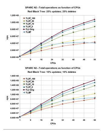
**Figure 3.** Throughput when private transactions do no work. A 2K sized Red-Black Tree on a 128 thread Niagara 2 with 25% puts and 25% deletes and 10% puts and 10% deletes for TL2, TL2-IP, and TL2P varying the percentage of private transactions: 100%, 50%, and 10%.
