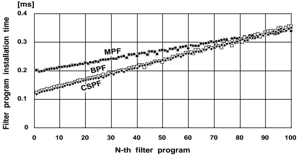
Figure 6: Filter program installation time, for the same protocol
