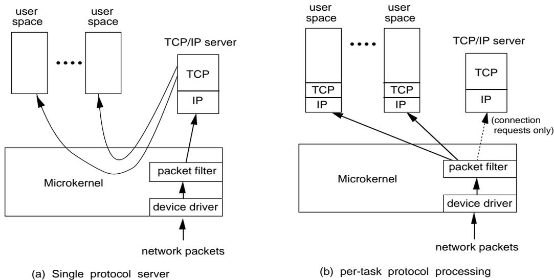
Figure 1: *Two ways to structure protocol processing. In the system on the left, all packets are routed through a central server and then on to their eventual destination. In the system on the right, the kernel routes an incoming, but unprocessed network packet directly to the address space for which the packet is ultimately intended.*
