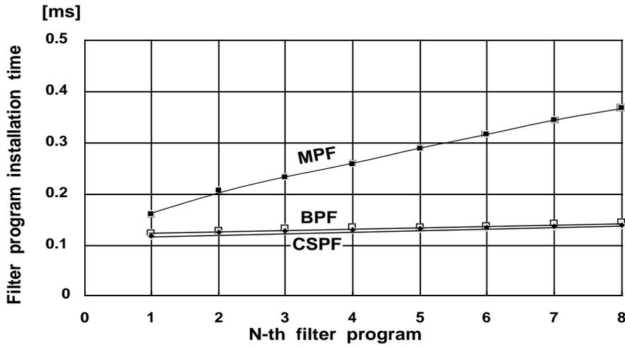
Figure 7: Filter program installation time, for different protocols.
