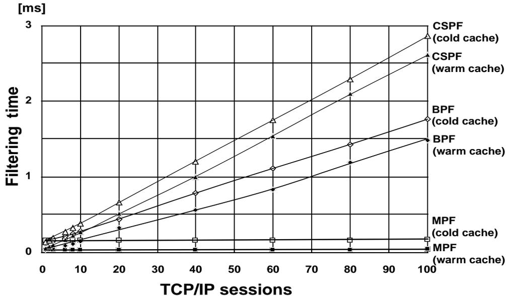
Figure 4: Filtering time of the three filter mechanisms
