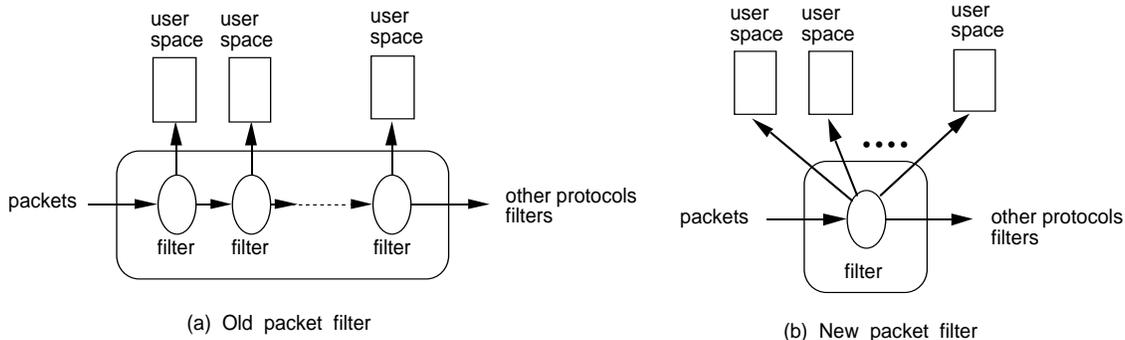
Figure 2: Redundant (BPF and CSPF) vs. one-step filtering (MPF) for incoming packets
