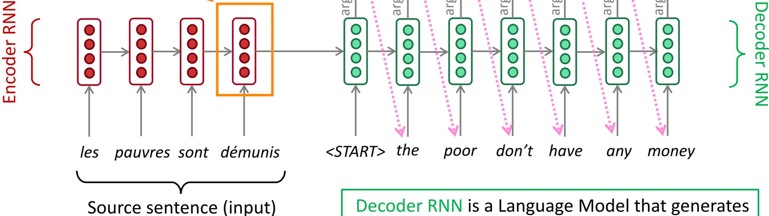
Encoder RNN produces an **encoding** of the source sentence.
