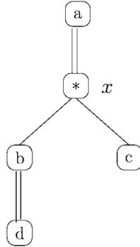
FIG. 1. A simple tree pattern with return node  $x$  marked. It corresponds to the XPath expression  $a// * [b//d][c]$ .
