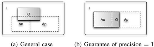
Fig. 5. Result relationship in Venn Diagram: The answer space is  $I$  (the Largest box) and the original answer are  $O$  (shaded box), the certain tuples in our model are  $A_c$ , the possible tuples is  $A_p$  (both are boxes with dotted-line).
