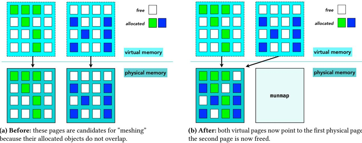
**Figure 1. MESH in action.** MESH employs novel randomized algorithms that let it efficiently find and then “mesh” candidate pages within *spans* (contiguous 4K pages) whose contents do not overlap. In this example, it increases memory utilization across these pages from 37.5% to 75%, and returns one physical page to the OS (via `munmap`), reducing the overall memory footprint. MESH’s randomized allocation algorithm ensures meshing’s effectiveness with high probability.
