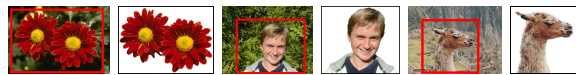
Figure 1: Three examples of GrabCut. The user drags a rectangle loosely around an object. The object is then extracted automatically.
