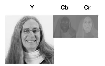
subsampled by a factor of 2 in each dimension, 4x size reduction on two of our three channels, reduces size by 1/2 overall
