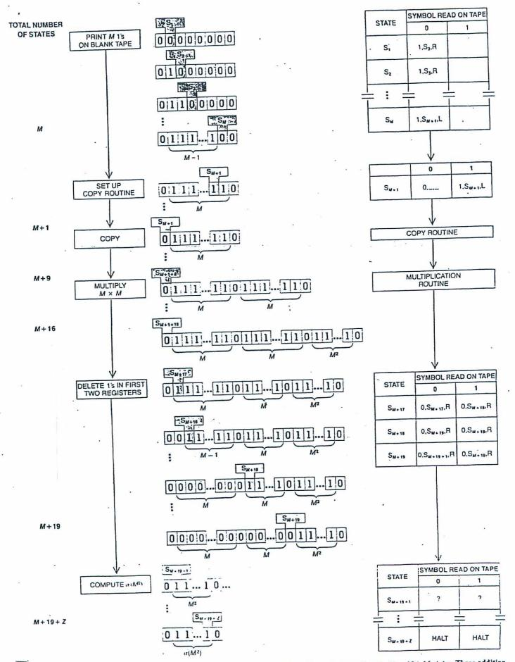
PROOF THAT  $\sigma(N)$  IS NONCOMPUTABLE begins with an estimate of the number of states needed to generate a string of  $M^2$  1's on a tape initially filled with 0's. The Turing machines for copying and multiplying, shown in the illustrations on pages 89 and 91, are
