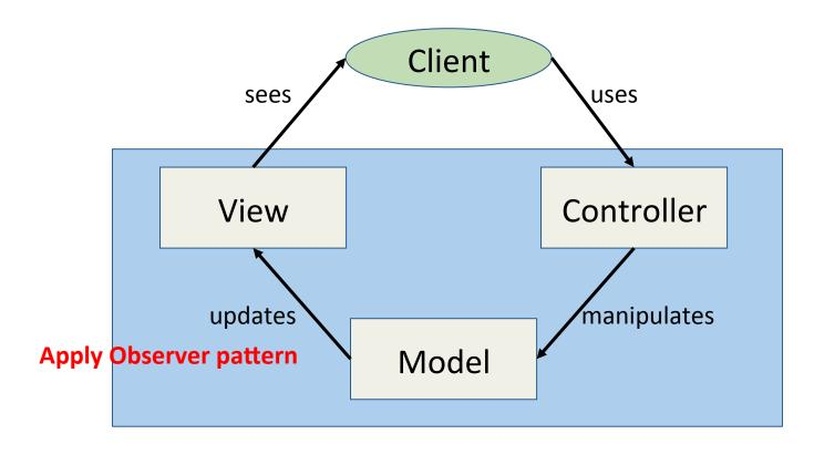
Separates data representation (Model), visualization (View), and client interaction (Controller)
