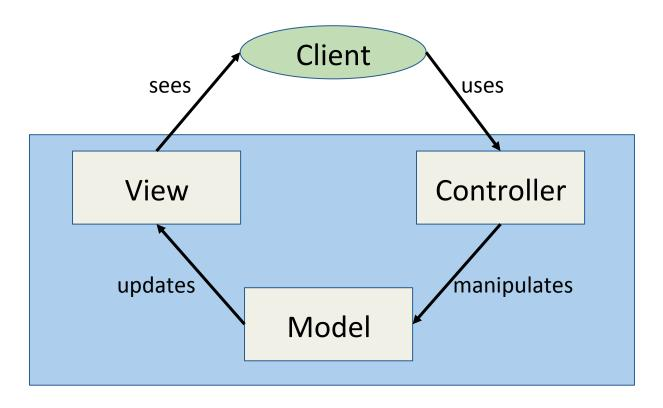
Separates data representation (Model), visualization (View), and client interaction (Controller)
