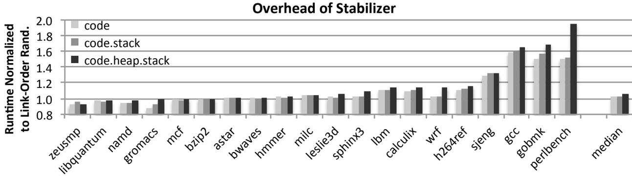
**Figure 3.** Overhead of STABILIZER relative to runs with randomized link order. With all randomizations enabled, STABILIZER adds a median overhead of 5.5%, below 20% overhead for 16 of 20 benchmarks, and in five cases slightly improves performance.
