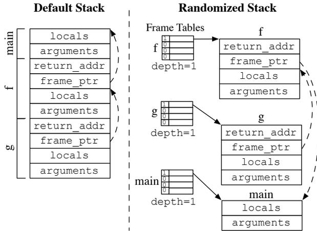
**Figure 2.** STABILIZER makes the stack non-contiguous. Each function has a frame table, which stores a frame for each recursion depth.
