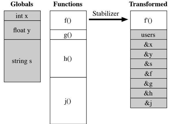
**Figure 1.** STABILIZER adds a relocation table to the end of each function, making every function independently relocatable. White boxes contain code and shaded boxes contain data.
