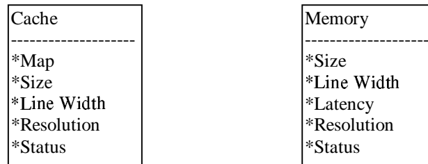
Figure 2 – Object Definitions of Cache and Memory Components
