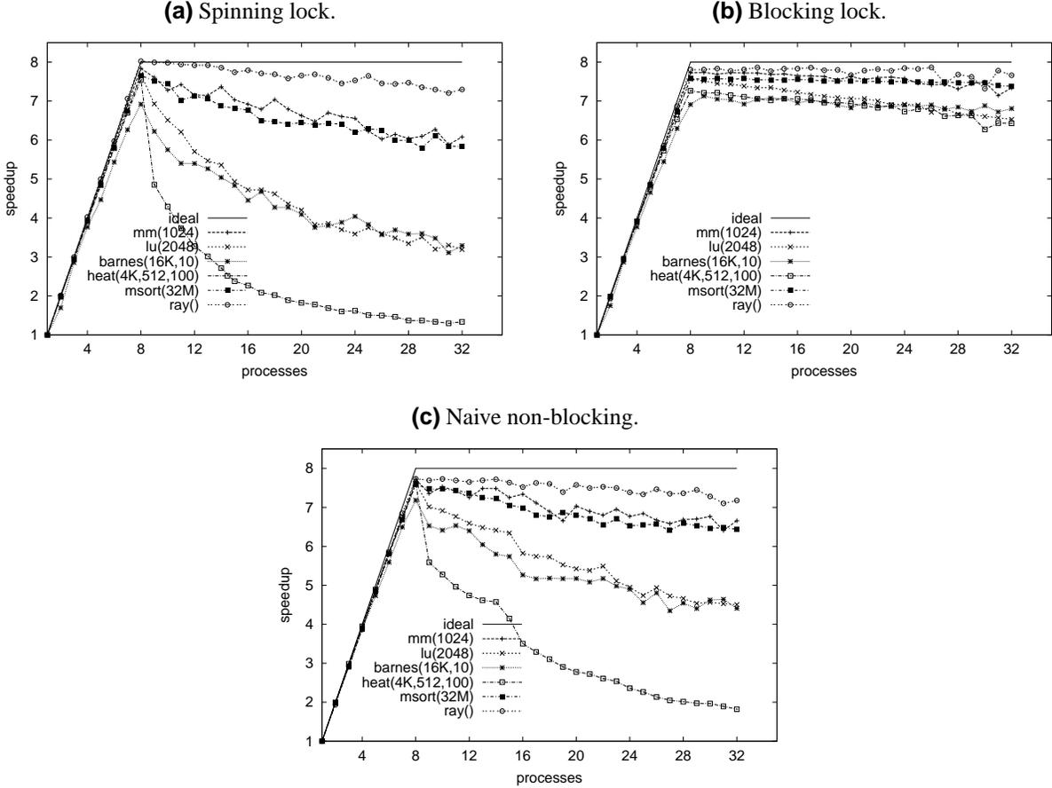
**Figure 2:** The speedup of work-stealing applications plotted as a function of the number  $P$  of processes when run on a dedicated 8-processor machine, for the three alternative implementations of work stealing.
