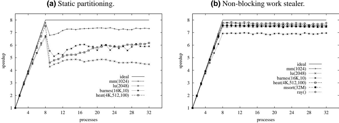
**Figure 1:** Measured speedup plotted as a function of the number  $P$  of processes used when run on a dedicated 8-processor machine. **(a)** Measured speedup for statically partitioned applications. **(b)** Measured speedup for work-stealing applications using the non-blocking work stealer.
