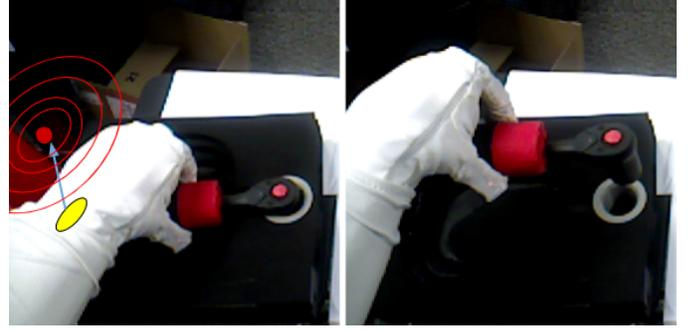
Fig. 2. Example of a *robot-proprioceptive action* ( $a_{RP}$ ) that extracts the ratchet.
