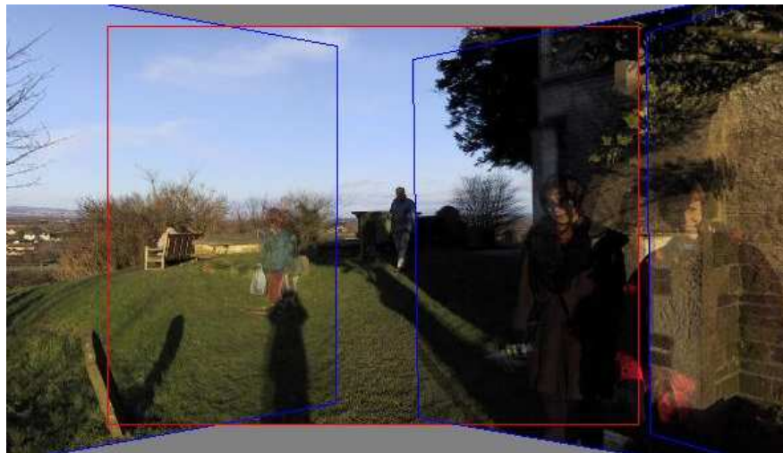
Figure 20: Validation of image matches by direct pixel error comparison can fail when the scene contains moving objects.
