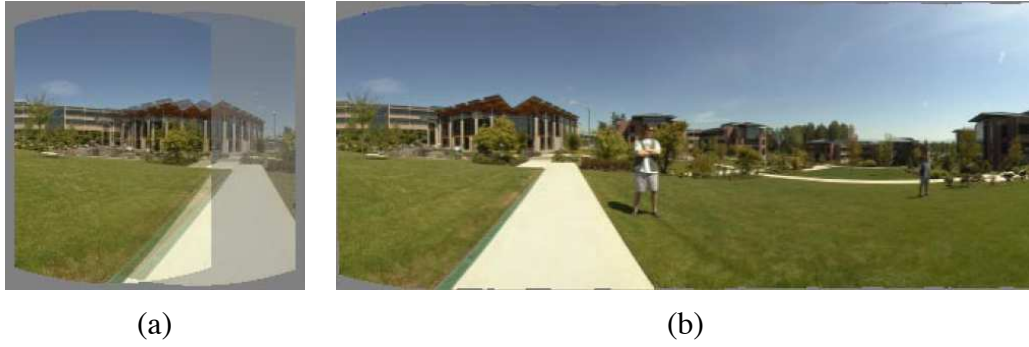
Figure 7: An example of a cylindrical panorama: (a) two cylindrically warped images related by a horizontal translation; (b) part of a cylindrical panorama composited from a sequence of images.
