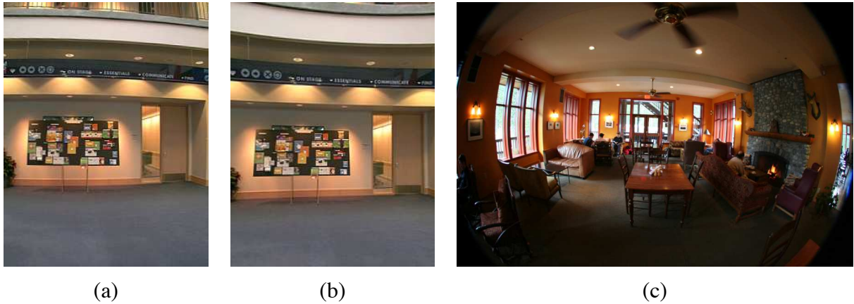
Figure 9: Examples of radial lens distortion: (a) barrel, (b) pincushion, and (c) fisheye. The fisheye image spans almost a complete 180^\circ from side-to-side.
