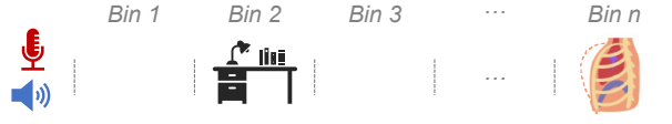
Fig. 3. The chirp signal allows us to separate the reflections from different distances into multiple range bins. The fine-grained activities can be extracted from the signal variations caused by the target movement (e.g., respiration) within a range bin.
