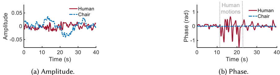
Fig. 11. The signal amplitude variation for the static object (chair) is relatively large, but its signal phase variation is quite small. The human motions can induce a much larger signal phase variation.
