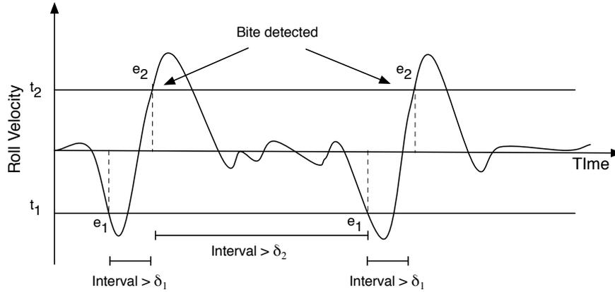
Fig. 8 BiteCounter [6] observes a sequential pattern of threshold-crossing events in the roll-velocity of a wrist to detect a food-intake gesture. The thresholds  $t_1, t_2, \delta_1, \delta_2$  are learnt empirically.
