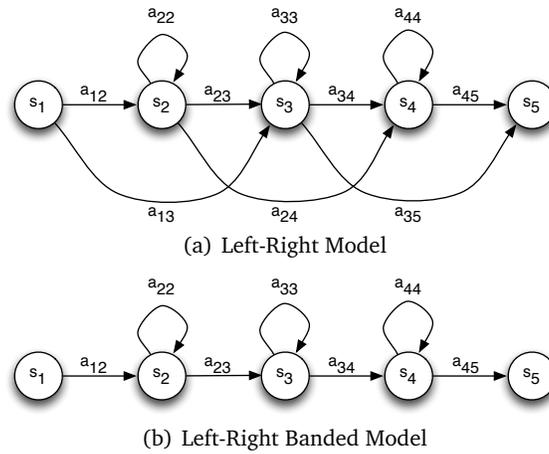
**Fig. 7** Left to Right HMM models are a popular choice for gesture recognition due to the temporal ordering of sub-gestures observed in a hand gesture.  $a_{ij}$  gives the probability of state transition from  $s_i$  to  $s_j$ .
