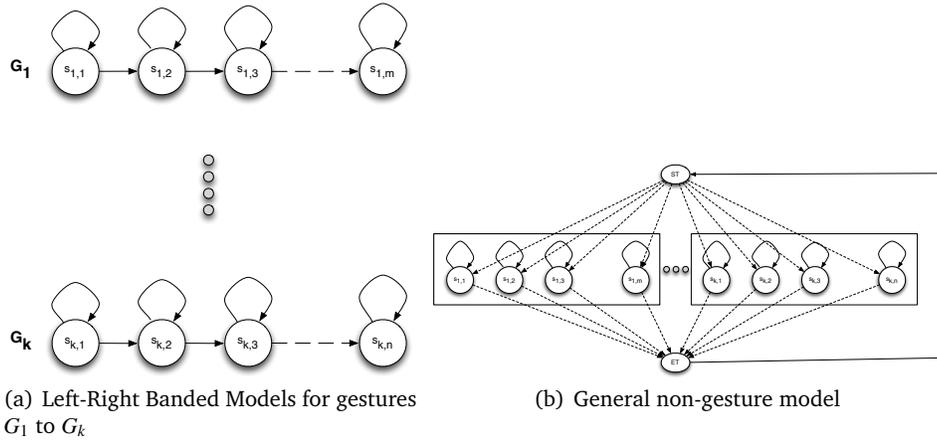
**Fig. 11** A non-gesture model constructed using the gesture models.  $ST$  and  $ET$  are the start and the end dummy states respectively.
