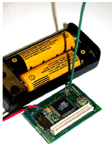
Fig. 3. The Rene Mote: a hardware platform for wireless networking
