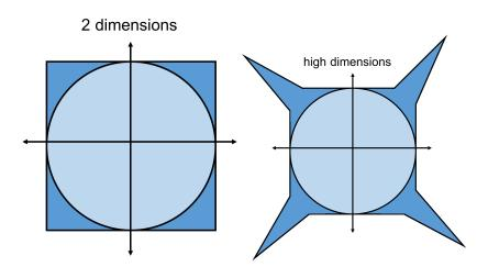
Corners of cube are  $\sqrt{d}$  times further away from the origin than the surface of the ball.
