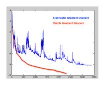
$$\vec{\theta}^{(i+1)} = \vec{\theta}^{(i)} - \eta \cdot \vec{\nabla} f_{j_i}(\vec{\theta}^{(i)}) \text{ vs. } \vec{\theta}^{(i+1)} = \vec{\theta}^{(i)} - \eta \cdot \vec{\nabla} f(\vec{\theta}^{(i)})$$
