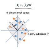
Claim: If  $\vec{x}_1, \dots, \vec{x}_n$  lie close to a k-dimensional subspace  $\mathcal{V}$  with orthonormal basis  $\mathbf{V} \in \mathbb{R}^{d \times k}$ , the data matrix can be approximated as:
