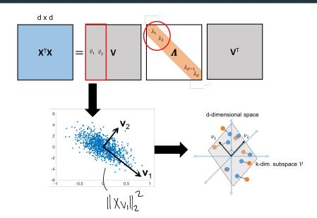
**Upshot:** Letting  $V_k$  have columns  $\vec{v}_1, \dots, \vec{v}_k$  corresponding to the top k eigenvectors of the covariance matrix  $X^TX$ ,  $V_k$  is the orthogonal basis minimizing
