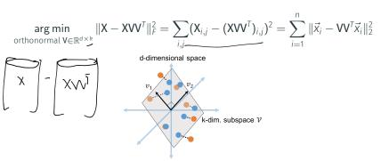
If  $\vec{x}_1, \dots, \vec{x}_n$  are close to a k-dimensional subspace  $\mathcal{V}$  with orthonormal basis  $V \in \mathbb{R}^{d \times k}$ , the data matrix can be approximated as ||X;||<sup>2</sup> = ||X;\/\r\x;||<sup>2</sup>  $XVV^T$ . XV gives optimal embedding of X in V.
