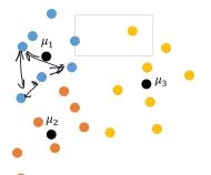
k-means Objective:  $Cost(C_1, \ldots, C_k) = \min_{C_1, \ldots, C_k} \sum_{j=1}^{\kappa} \sum_{\vec{x} \in C_k} \|\vec{x} - \mu_j\|_2^2.$
