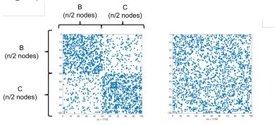
$G_n(p,q)$ : stochastic block model distribution. B,C: groups with n/2 nodes each. Connections are independent with probability p between nodes in the same group, and probability q between nodes not in the same group.
