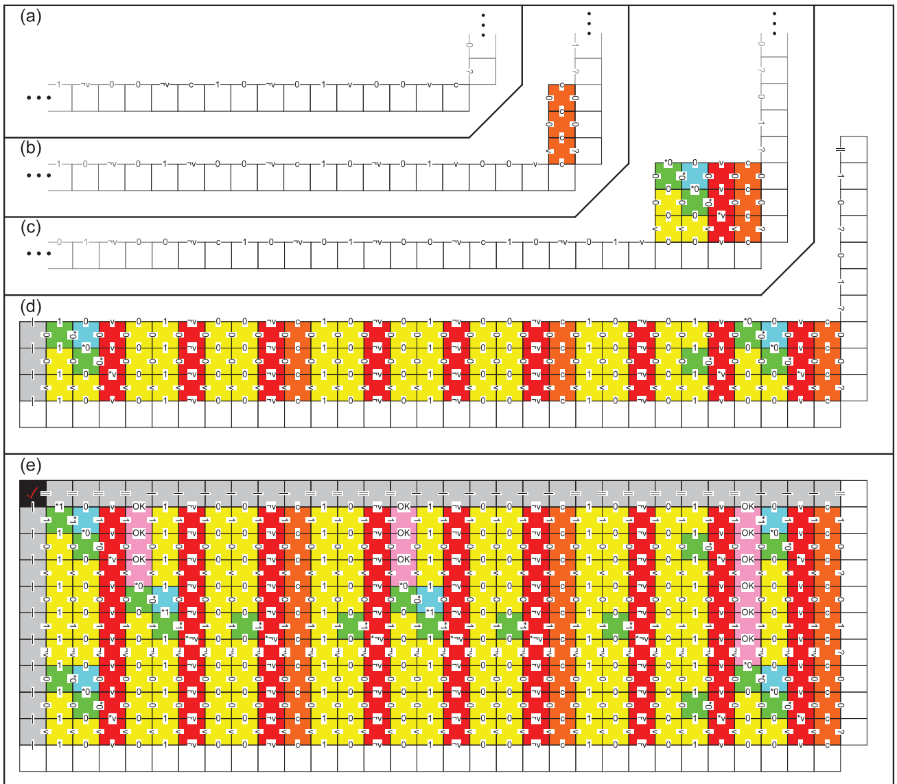
Fig. 4. An example progression of the growth of a crystal of the 3-SAT-solving tile assembly. The crystal seed (a) consists of the clear seed tiles, encoding the input \phi = (x_2 \vee \neg x_1 \vee \neg x_0) \wedge (\neg x_2 \vee \neg x_1 \vee \neg x_0) \wedge (\neg x_2 \vee x_1 \vee x_0) . Specially designed tiles (Fig. 3) attach to nondeterministically select a variable assignment for x_0 (b); compare that assignment to, first, a single literal in \phi (c); and then, the rest of the literals in \phi (d); and, finally, repeat those steps for variables x_1 and x_2 and ensure that each clause is satisfied at least once by the particular selected variable assignment (e). Because \phi is satisfied when x_0 = x_2 = \text{TRUE} and x_1 = \text{FALSE} , represented by the tiles in the second from the right column in (e), the black \checkmark tile attaches in the top left corner.
