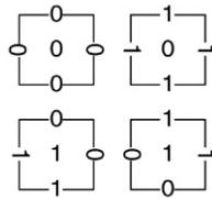
Fig. 5. A set of tiles that performs a left-shift on a row of 0s and 1s. In binary, a left-shift is a multiplication by 2.
