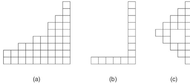
Fig. 1. A step-configuration (a), an L-configuration (b), and a configuration that is neither a step-configuration nor an L-configuration (c). A step-configuration has no holes and consists of a finite number of consecutive rows, such that each row has the same rightmost position and is shorter than the row below it. An L-configuration is a special case of a step-configuration and looks like the mirror image of the letter L.
