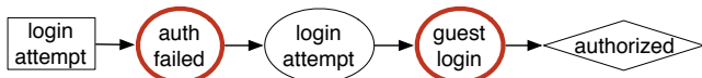
Figure 5: A path through the initial model in Figure 4(a) that violates the mined auth\ failed \not\rightarrow guest\ login invariant.
