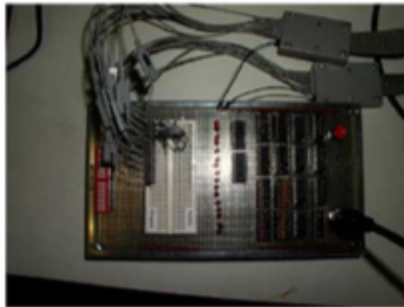
Wire wrapped circuit for quick evaluation of system dynamics.
