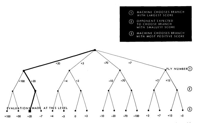
Figure 2 Simplified diagram showing how the evaluations are backed-up through the "tree" of possible moves to arrive at the best next move. The evaluation process starts at (3).
