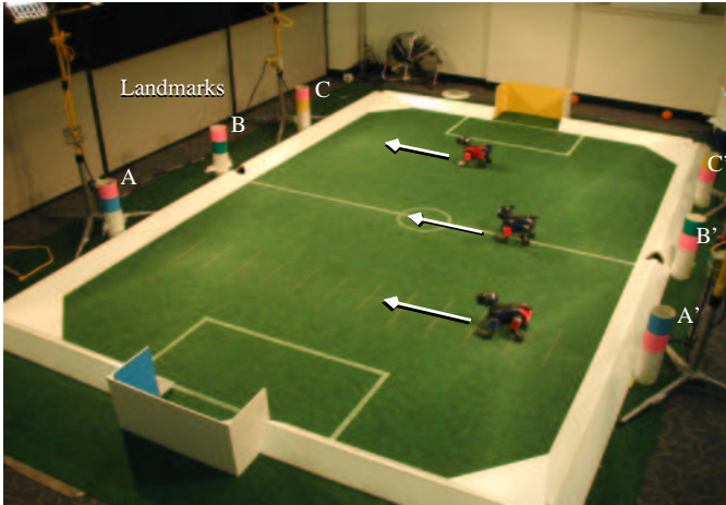
Fig. 5. The training environment for our experiments. Each Aibo times itself as it moves back and forth between a pair of landmarks (A and A', B and B', or C and C').
